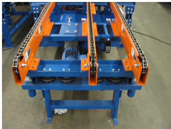
CHAIN TRANSFER END VIEW
