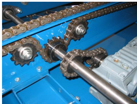
DRIVE SHAFT AND TAKE UP ARRANGEMENT SHOWN WITHOUT CDLR ROLLERS
