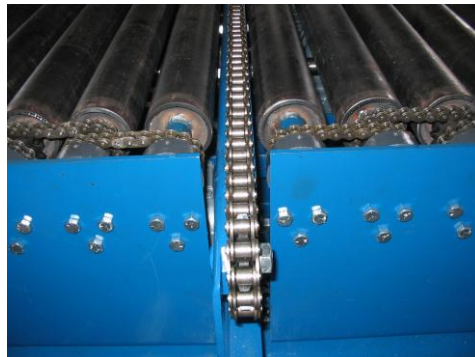
CONVEYOR CHAIN POSITIONED ON LIFT MECHANISM
